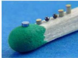
Resonators and non-reciprocal components sets for extremely high frequency engineering from any ferrite or dielectrics at measurements from >0,3 mm with tolerances to about 1  $\mu$ m. diameters
