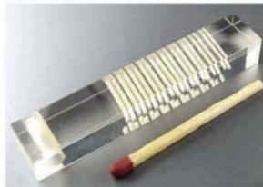
Sample of Zerodur with 20 Holes, Diameter 0,7 mm in a Angle von 10°.
