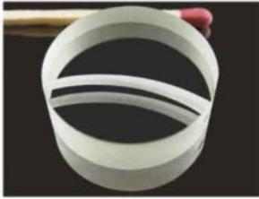
By the ultrasonic processing, boring arc-shaped in special cases of application can be set up as shown at the opposite. The sectional view can be provided with an almost any section.
