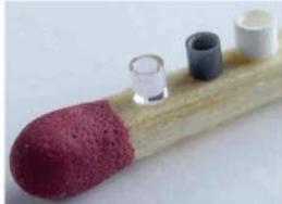
Cups and toecaps with spheric ground of AlN, Al<sub>2</sub>O<sub>3</sub>, SiC, Si<sub>3</sub>N<sub>4</sub>, Sapphire, Boronnitride and Silica. Sample:  $\phi$  1,5 mm, Lenght 1,4 mm, Wall-thickness > 0,2 mm.
