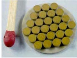
Piezo arrays. The size of the individual fields in the honeycomb shaped order is freely definable from about 0,5 mm. Processing can occur optionally of one or from two pages.
