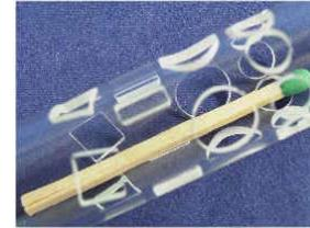
Glass tube diameter 16 mm, with ruptures profiled differently, partially tangentially to the inner surface.
