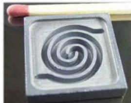
Complex parts from monocrystalline materials, for example, we process silicon with one, the form of ultrasonic processing engineering similar to CNC processing.
